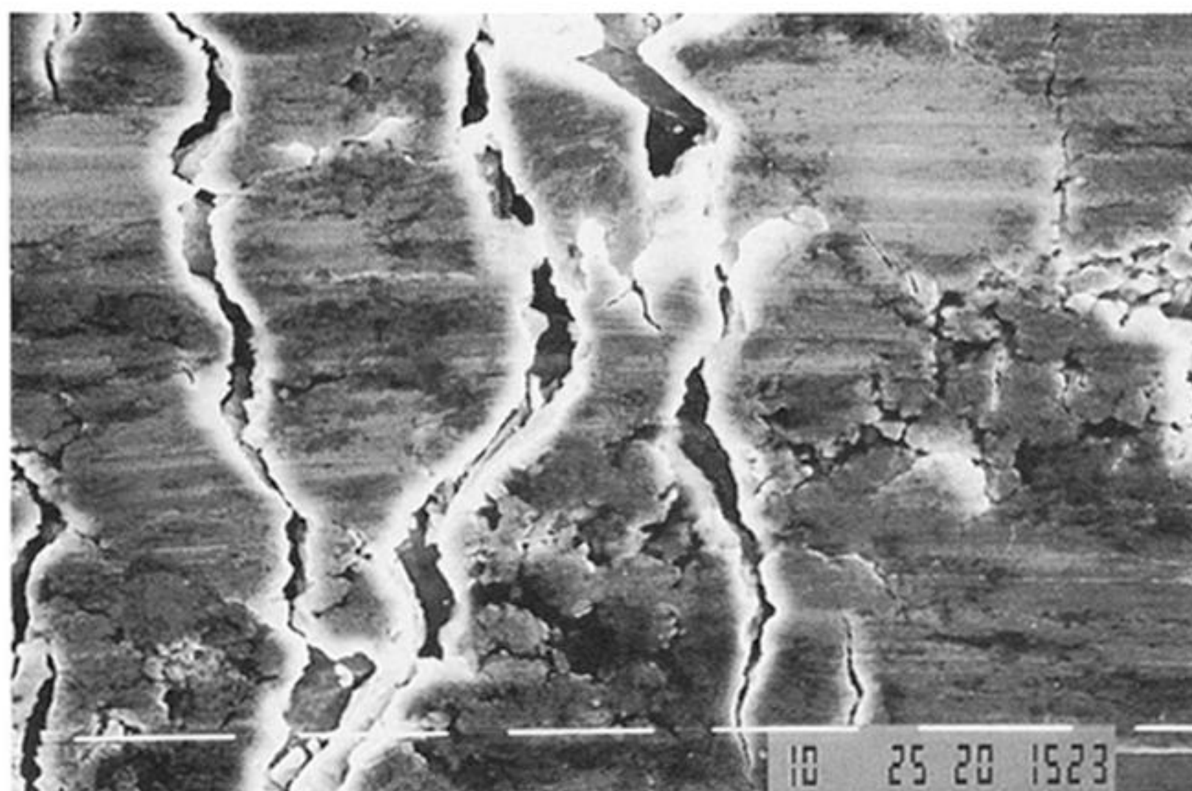
Figure 3. Galvannealed steel sheet: wall portion of hat channel product obtained under severe friction condition (degreased). SEM micrographs: (a) Cross section \times 500 , (b) outer surface \times 500 and (c) outer surface \times 1500 .
